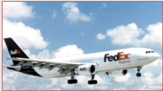
The new FedEx Airbus, with a length of 153 feet and a wingspan of 144 feet, will be able to transport nearly 50% more cargo than the Boeing 727.
